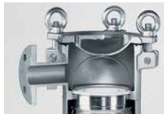
Compression bag hold down creates 360 degree sealing between filter bag and bag filter housing
