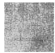
60 MESH Wire Dia. 0.0065 Opening 0.010 38% Open Area
