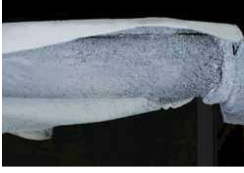
Filter element from an e-coat tank filtration after being in service for eleven weeks
