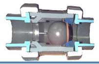
pressure moves the solid plastic ball off of the EPDM or FKM seat. When flow stops, the system back pressure pushes the ball against the seat stopping the flow. The ball is free floating, so it never seats twice in the same position, preventing uneven wear. Key features compared to competing designs are: the ball is retained with the true union nuts removed and it is safety blocked.
