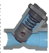
that benefit from quicker closure. For example, a spring assisted Y check valve would be a better choice for a viscous liquid than a ball check valve, especially if the system pressure is low. The Y design enables servicing in-line without the necessity of disrupting the pipeline connection or having a true union connection.
