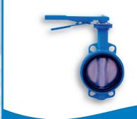
The Wafer Butterfly Valve is available with various disc and seat material variations to suit a wide range of applications. It should be installed with its shaft horizontal, lower edge of disc opening downstream.
